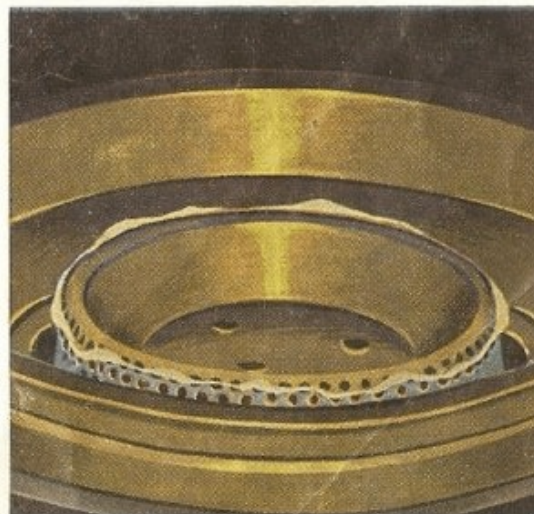
C. Turn wick up until a completely blue flame is obtained
